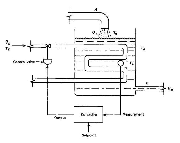
Inputs to the controller are measured indication of both the controlled variable & the set point expressed in the same fashion.
